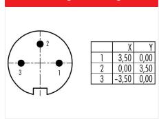
Contact arrangement (Plug-in side)
